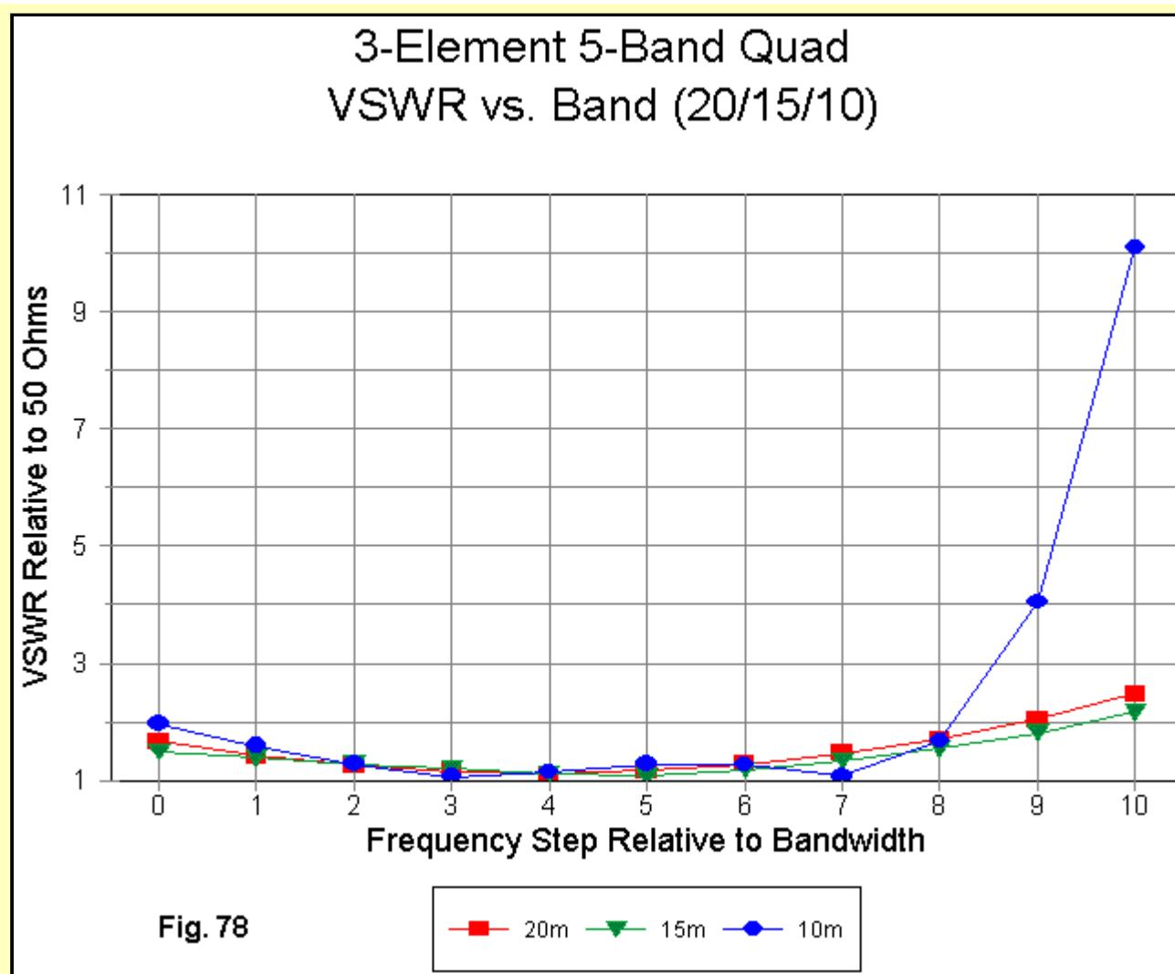
The small adjustments to the lower bands yield 50-Ohm SWR curves (Fig. 78) that are below 2:1 for 90% of 20 and 15 meters. The 10-meter 2:1 curve has been extended to over 80% of the pass band and is consistent with the patterning of the gain and front-to-back figures. 28.8 to 29 MHz has been sacrificed for optimized performance at the low and middle regions of the pass band. You may compare this figure with Fig. 74 to more clearly see the improvement in the 50-Ohm SWR category.
