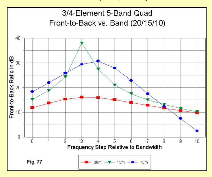
In **Fig. 77**, we can see the unchanged 15-meter front-to-back curve, which serves as a back drop for the other curves. 20 meters shows a movement of the curve to better center it within the band and give better upper band- edge performance. The biggest improvement occurs on 10 meters, where the front-to-back value is at least 15 dB for more than 3/4 of the pass band. As with the gain, we get a steep slope downward as the frequency approaches 29 MHz.
