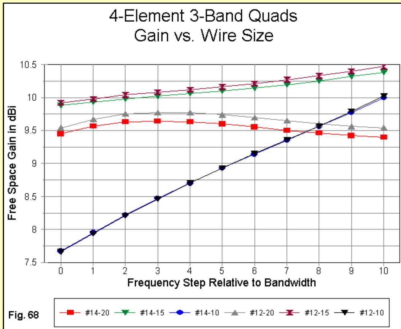
The gain curves in **Fig. 68** show the virtual identity of the 10-meter gain for the two wire sizes. 15-meter gain does almost as well, and only 20-meter gain shows something interesting. The low-end increase in gain toward the peak value is slightly steeper for the fatter wire.
