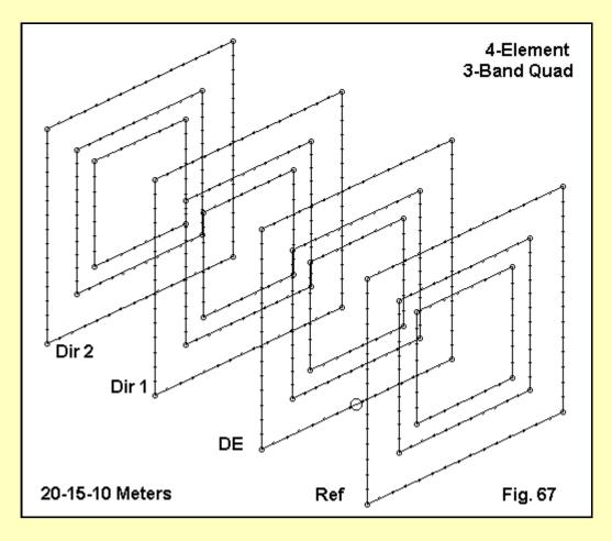
The following table lists the element lengths per loop side for each of the three bands.
