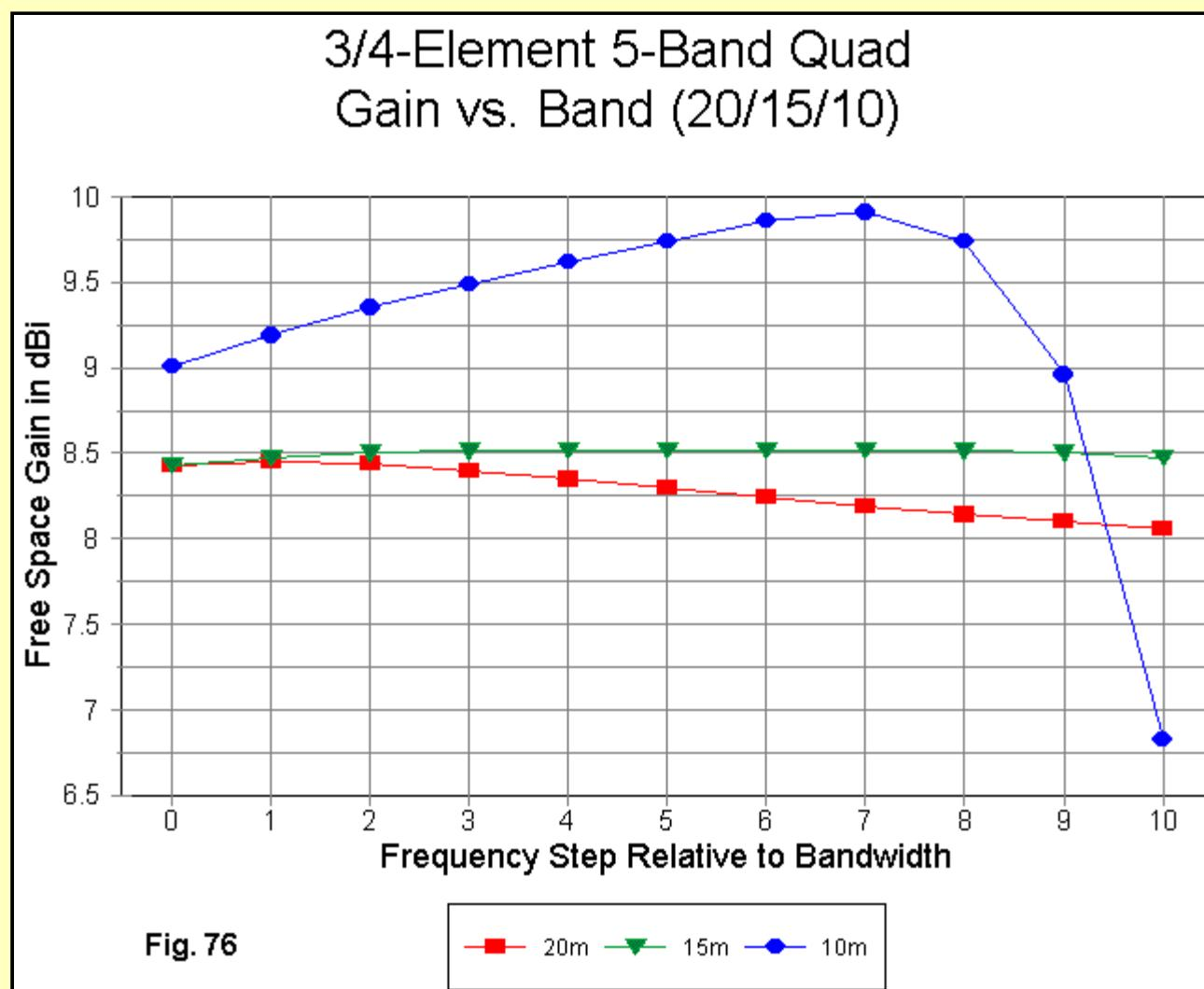
In the gain curves in **Fig. 76**, we may note that 15 remains unchanged in its flat curve, while the decrease in gain at the upper end of 20 meters has decreased. The gain curve for 10 meters remains at about 9 dBi or better for 90% of the pass band, before taking a nose dive.
