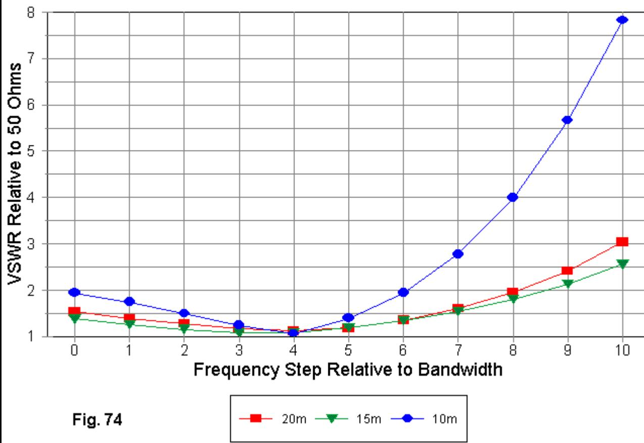
The 50-Ohm SWR performance of the antennas has also been optimized for the low ends of the bands, as is readily apparent in **Fig. 74**. On 20 and 15, the SWR is below 2:1 for at least 80% of the pass bands, but that figure goes down to 60% on 10 meters. For reference, here are the standard figures across each of the wide bands.
