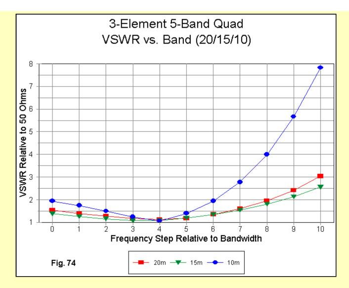
The 50-Ohm SWR performance of the antennas has also been optimized for the low ends of the bands, as is readily apparent in **Fig. 74**. On 20 and 10, the SWR is below 2:1 for at least 80% of the pass bands, but that figure goes down to 60% on 10 meters. For reference, here are the standard figures across each of the wide bands.
